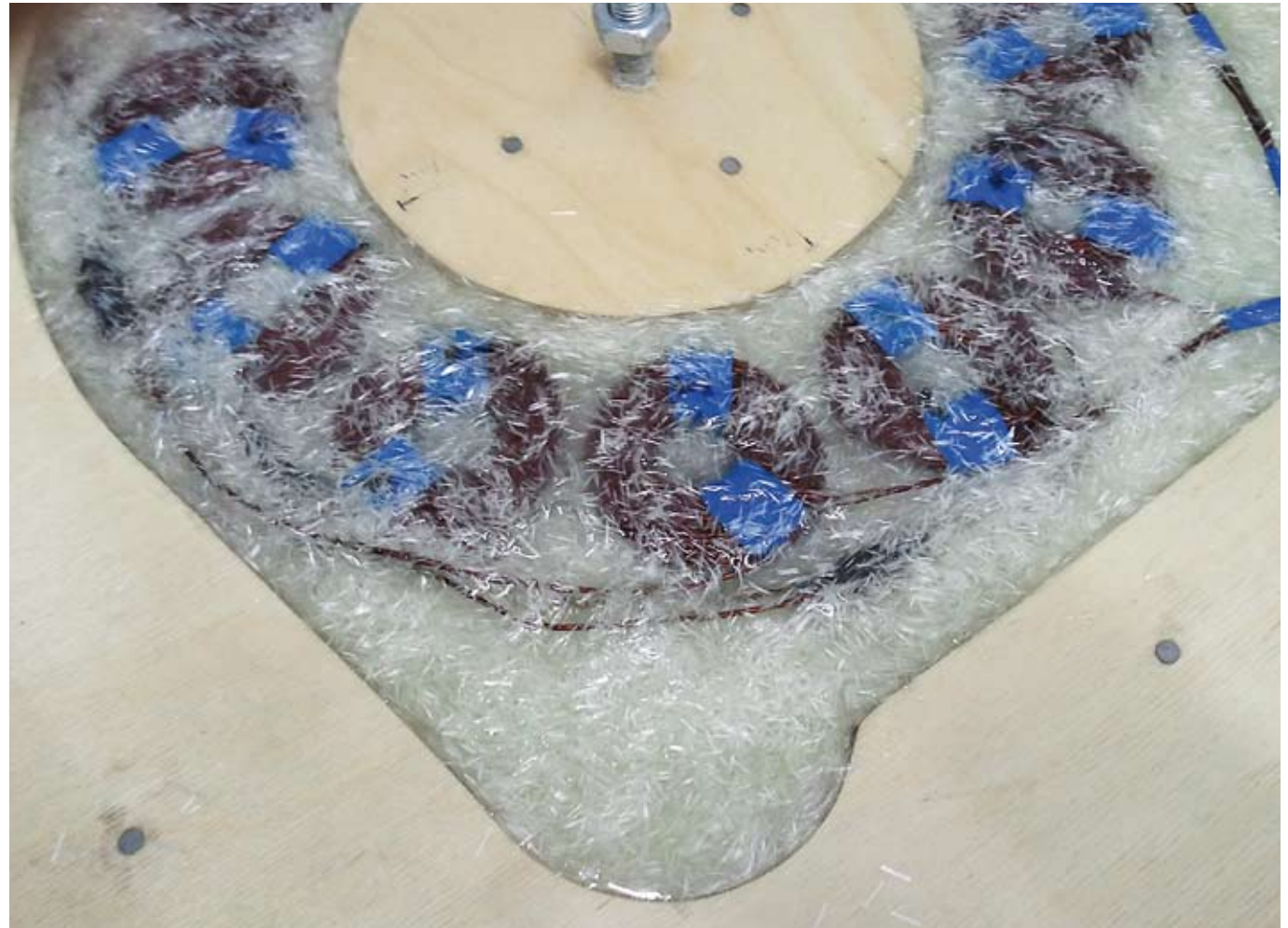
Abb. 23: in Epoxidharz gegossene Spulen
